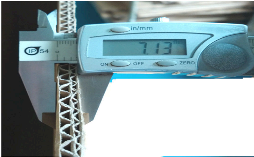
REACH outside box: Five layer corrugated cardboard 7mm thickness
